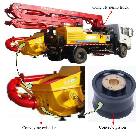
Figure 1. Concrete pump truck and concrete piston.
